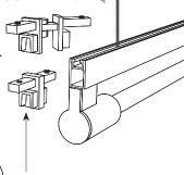
STJR-creates a mechanical connection for continuous runs. One connector is included with each two connecting fixtures.
